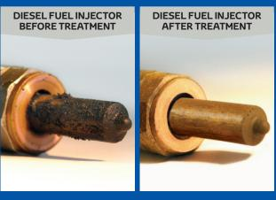
Just one treatment is all it takes to rid the diesel fuel injector of the deposits that impair performance.
